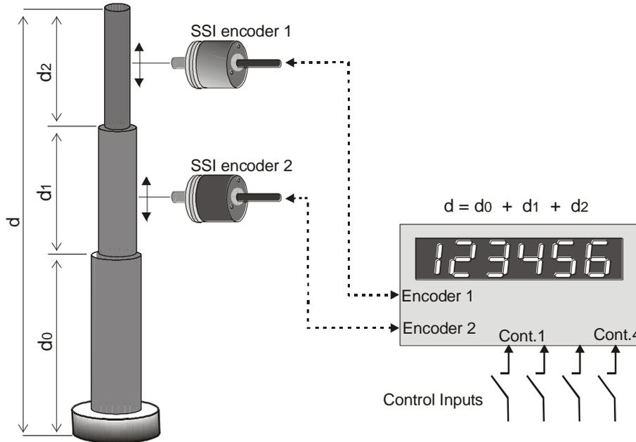
Both encoder inputs are connected to SSI encoders and the unit calculates the sum of positions of both encoders. The encoders may have different resolutions and can operate at different Baud rates and individual scaling. The result of the calculation (sum) can once more be converted to the desired engineering units by means of the final scaling parameters.
