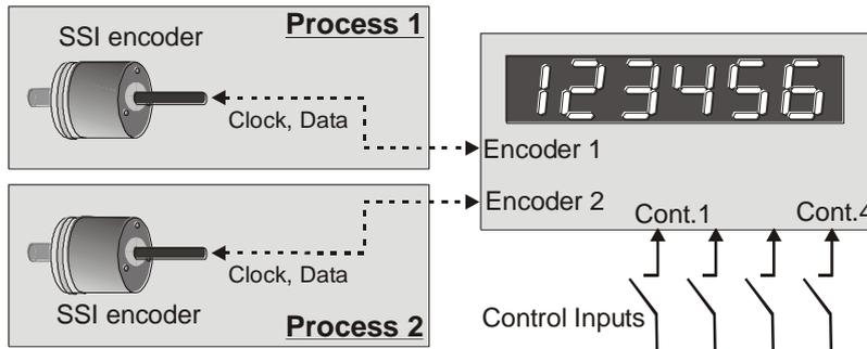
Both encoder inputs are connected to SSI encoders for individual evaluation. The encoders may have different resolutions and can operate at different Baud rates and individual scaling.
