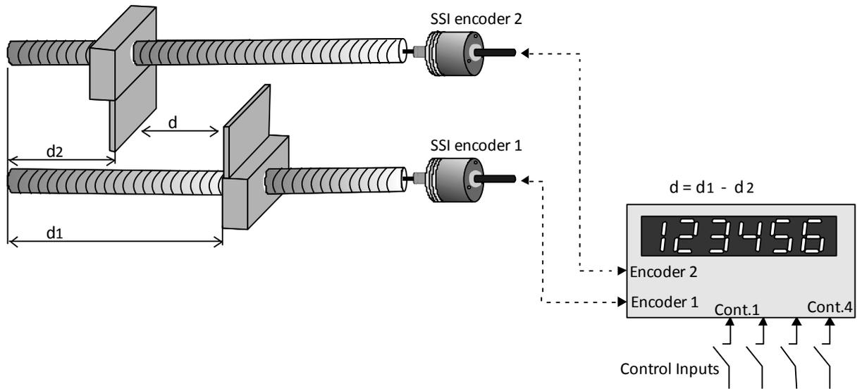
Both encoder inputs are connected to SSI encoders and the unit calculates the differential position of both encoders. The encoders may have different resolutions and can operate at different Baud rates and individual scaling. The result of the calculation (difference) can once more be converted to the desired engineering units by means of the final scaling parameters.
