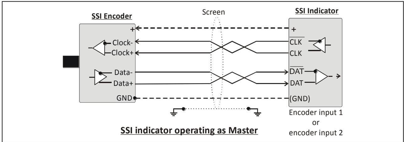
When the encoder already receives its clock from a remote unit and the SSI indicator should only "listen" to the communication, the corresponding encoder input must be configured as "Slave". In this case the clock terminals (CLK) of the indicator are configured as inputs.
